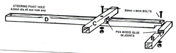
Fitting wheel brackets: Fix axle brackets to Part A and B,using screws/bolts as appropriate. Heads of bolts must be to the top side of Part D if used. Front wheel brackets must be positioned to allow rope holes on the forward part of Part A and so located that the axle position leaves pivot bolt and nuts accessible for adjustments.
